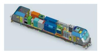
The carbody is designed to allow compression forces up to 3,5 MN (buff load = 800,000 lbs). It is equipped with a Crash Energy Managment (CEM) system that provides enhanced safety for the crews, consisting of an AAR F-Type coupler with pushback mechanism and crash elements.
